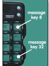
A blue LED indicates Function Mode is on. Press any labeled message key to select that setting. Red LEDs around the key will light when the setting is activated. Press the Exit key (bottom right on green membrane) to exit Function Mode.
