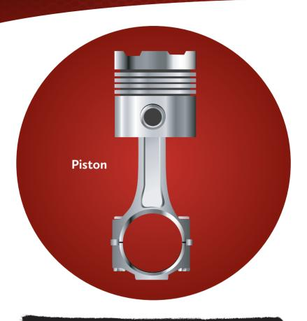
Each tube has a *piston*. The piston moves up and down.
